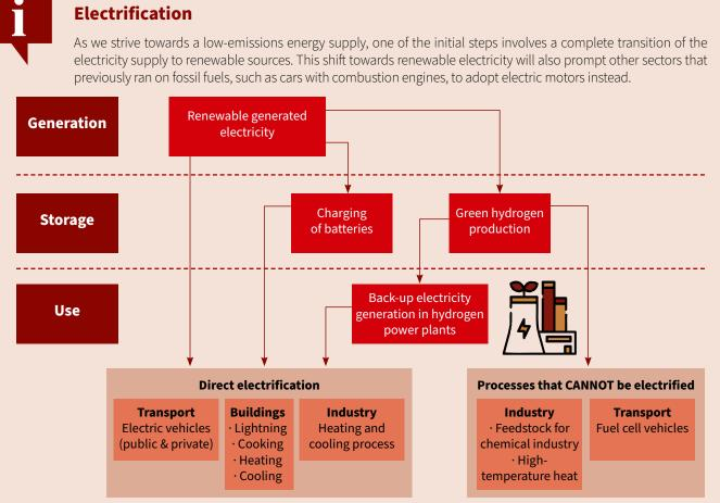
Processes that cannot be electrified directly can frequently be powered by hydrogen derived from renewable energy. By incorporating electricity generated from renewables into industrial processes, emissions from these processes can be either wholly averted or substantially reduced.<sup>4</sup>
